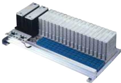
HART over Profibus functionality enables the HART information to be passed through the system direct to Asset Management Packages such as AMS Device Manager.
