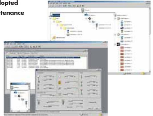
IMS products provide essential configuration, calibration, monitoring and maintenance history functions for conventional analog (4-20 mA) and HART protocol compatible smart process instruments and field devices. They deliver powerful tools to meet the need for standardised instrument maintenance procedures and record keeping mandated by some quality standards and regulatory bodies.
