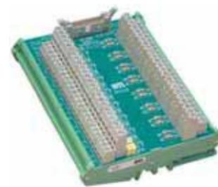
The HART multiplexer is the brains of the system. Its is a combination of two modules, the MTL4841 - HART communications module and MTL4842 - HART interface module. They provide the HART data interface between smart devices in the field and HART instrument management software running on a PC. The modules which mount on the BPHM64 HART backplane connect to the field devices via either HART connection units or IS backplanes depending on the application.
