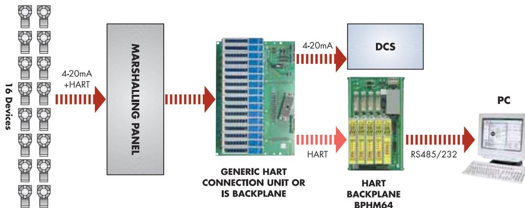
The MTL4840 system is however completely modular and scalable allowing you to grow the system to the size you require. i.e each 16 channel HART connection board is connected to one MTL interface module and up to 16 of these modules can be connected to one HART communications module. This enables one multiplexer to communicate with up to 256 different HART devices in the network. Additionally up to 31 HART Comms modules can be daisy linked giving 7936 HART devices on one network.
