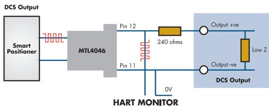
In IS applications, fitting a simple resistor between the output +ve and the input to the isolator will raise the impedance up to the required level. In some cases it may be necessary to add additional filtering between the output and the isolator if:
