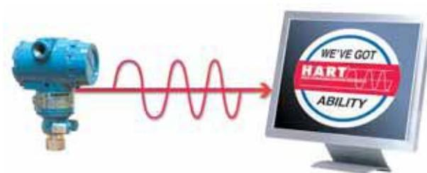
*The HART protocol allows additional information to be carried on the same pair of wires with the 4-20mA analogue signal.*
