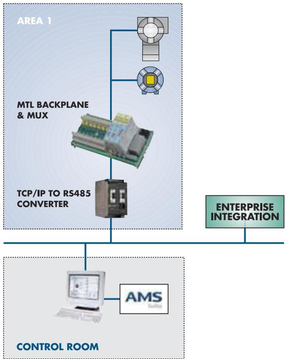
HART devices on the manned platform were connected via the HART backplanes to the copper RS485 network. All HART devices on manned and unmanned platforms were now connected to the serial port on one PC running Cornerstone software. This enabled all devices to be monitored and configured without the need for an engineer to visit the unmanned platform.
