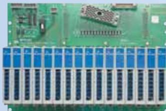
HART data is routed from each isolator via a 20-way ribbon cable to the MTL4842 HART multiplexer mounted on the backplane.
