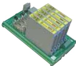
The HART backplane is the backbone of the MTL4840 system. This small but vitally important board holds the MTL4840 HART modules which handle the HART multiplexing. Each board can communicate with up to 64 HART devices.
