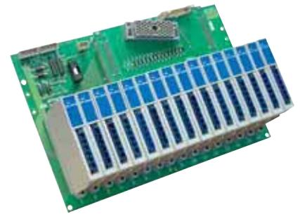
**MTL4000 Series backplanes provide both mechanical and electrical connections through the backplane. The advantages they offer include:**
